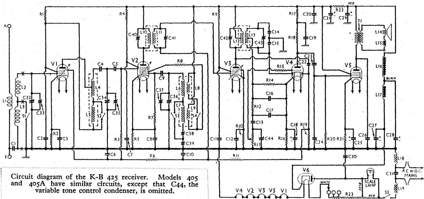
Circuit diagram of the K-B 425 receiver. Models 405 and 405A have similar circuits, except that C44, the variable tone control condenser, is omitted.
