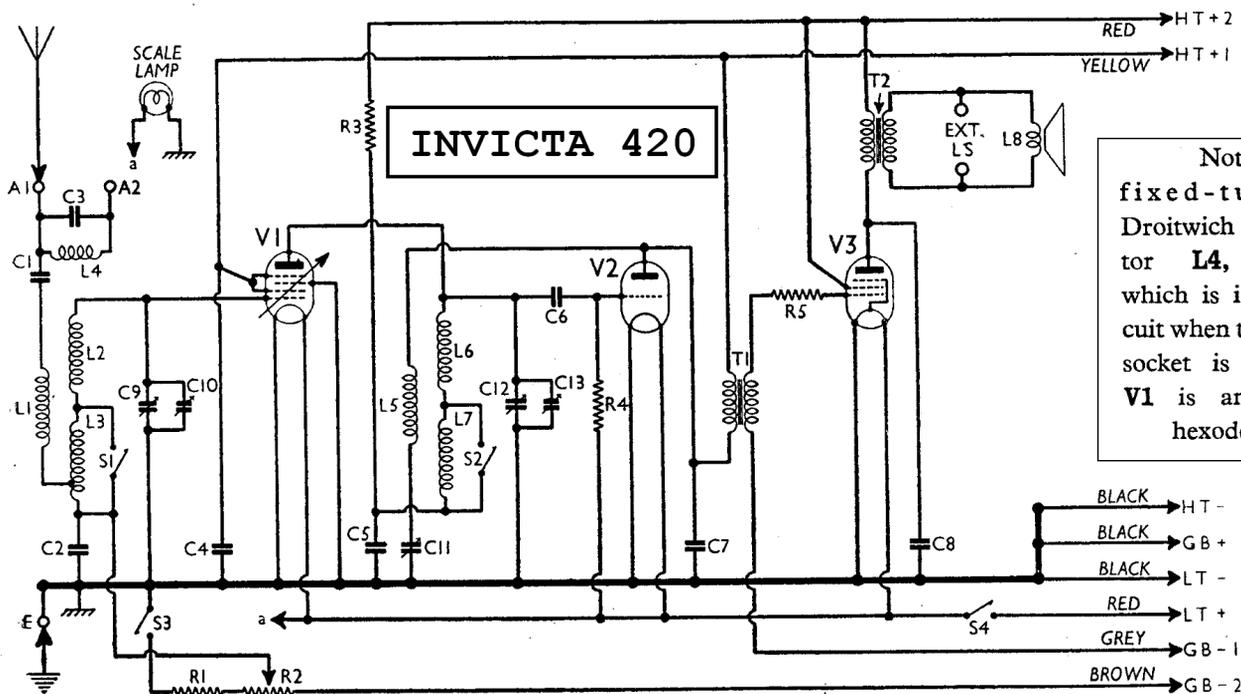
Note the fixed-tuned Droitwich rejector **L4, C3**, which is in circuit when the **A2** socket is used. **V1** is an RF hexode.
