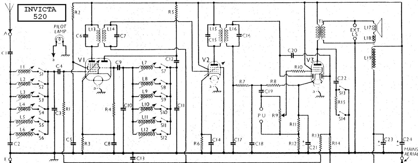
No manual tuning is provided in the Invicta 520 AC superhet, but press-buttons give the choice of any of six stations, and operate on the permeability system. When the mains aerial is not in use **C25** is earthed and acts as a mains RF by-pass.
