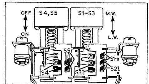
Switches S1-S5 as seen when viewed from the front of an upright chassis. The buttons depress and release independently giving two switch position for each button.
