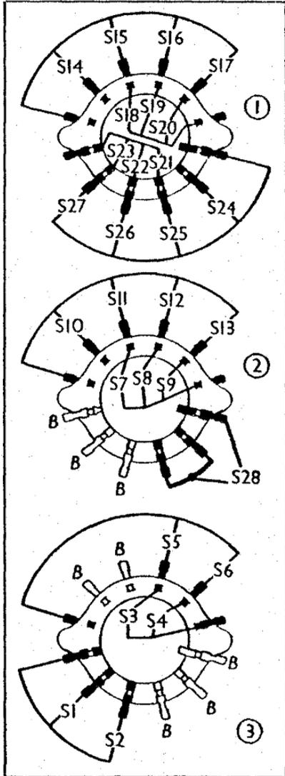
**MW.**—Connect signal generator via a dummy aerial or 0.0005  $\mu$ F condenser to A socket, and E. Switch to MW, tune to small white dot on scale between the 210 and 220 m calibrations, inject a 1,400 KC/S (214.3 m) signal and adjust C42, C30 and C34 for maximum output, using the T.I. as a visual indicator.
