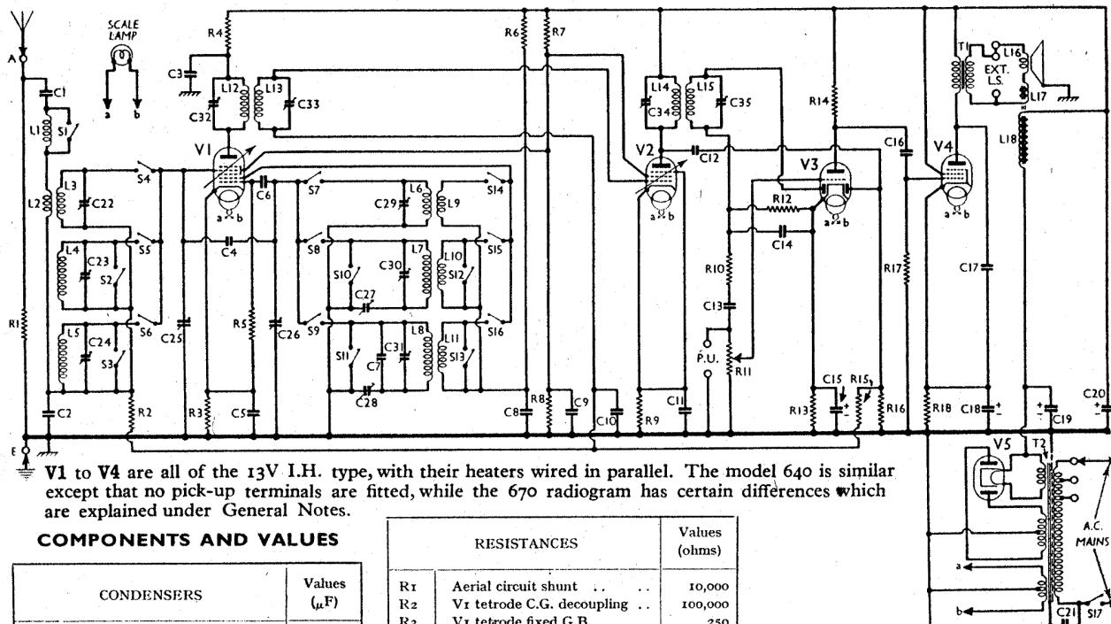
V1 to V4 are all of the 13V I.H. type, with their heaters wired in parallel. The model 640 is similar except that no pick-up terminals are fitted, while the 670 radiogram has certain differences which are explained under General Notes.
