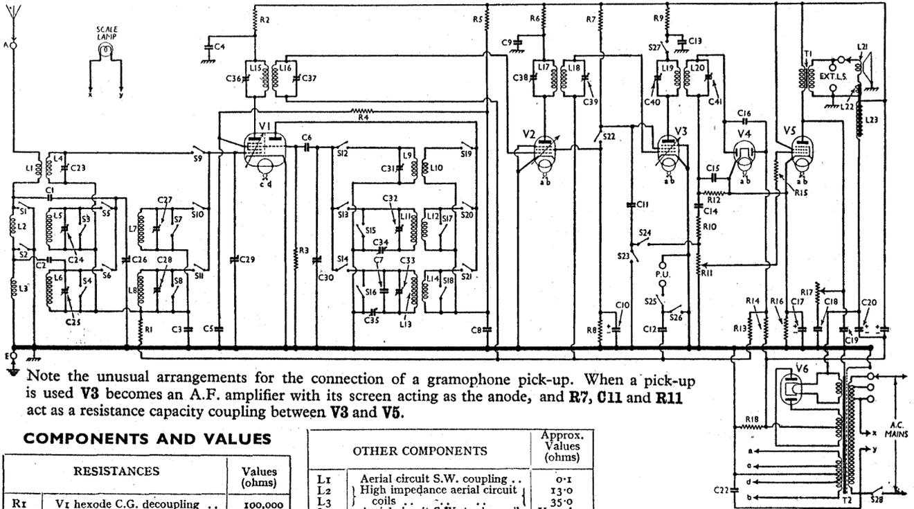
Note the unusual arrangements for the connection of a gramophone pick-up. When a pick-up is used V3 becomes an A.F. amplifier with its screen acting as the anode, and R7, C11 and R11 act as a resistance capacity coupling between V3 and V5.
