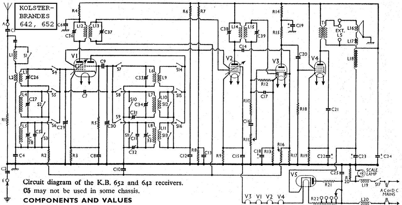
Circuit diagram of the K.B. 652 and 642 receivers.
