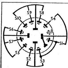
Diagram of the S1-S10 switch unit, seen from the rear. Below is the associated switch table.
