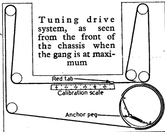
approximately mid-scale positions, and adjust the cursors as necessary. On M.W. and L.W. it may be necessary to set the cursor to give the best compromise on both wavebands.
