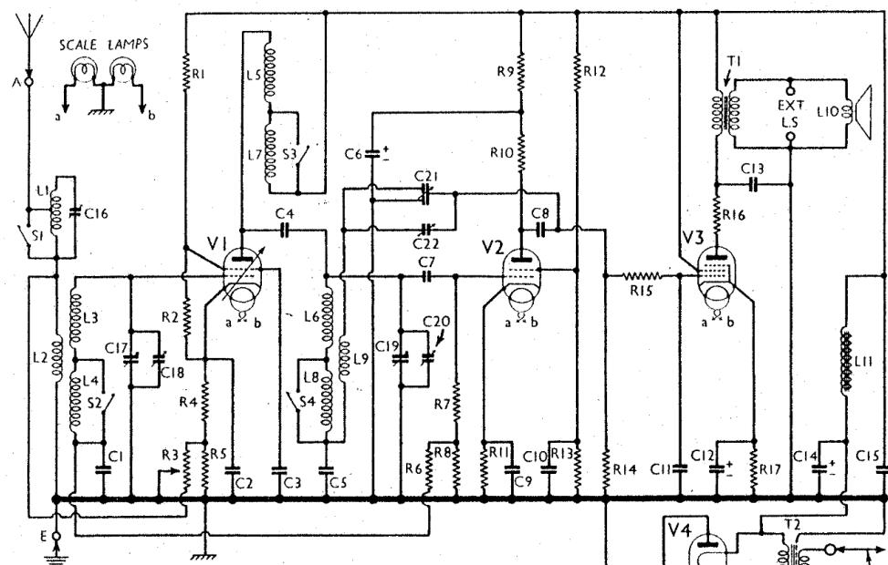
Circuit diagram of the G.E.C. AC37 receiver. Note the arrangement for biasing **V1** from the grid circuit of **V2**.
