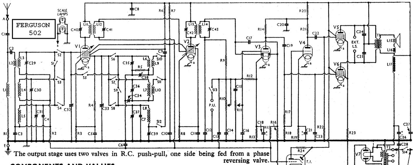
The output stage uses two valves in R.C. push-pull, one side being fed from a phase reversing valve.
