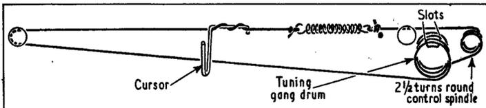
Sketch of the drive cord system as seen from the front of the chassis.
