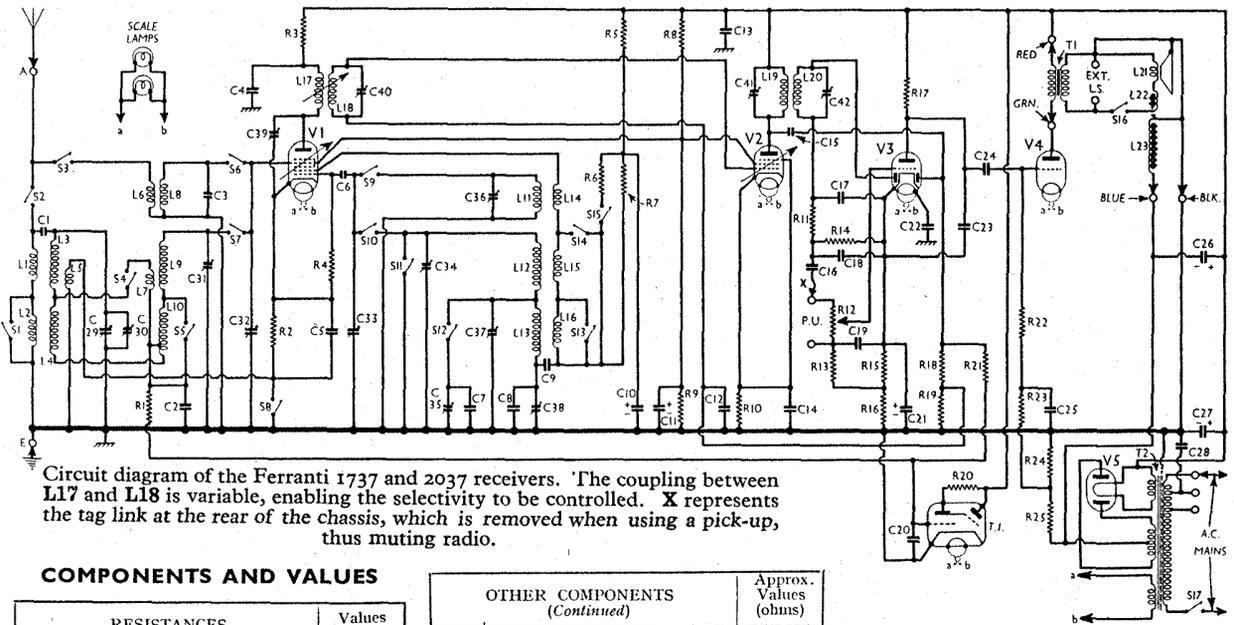
Circuit diagram of the Ferranti 1737 and 2037 receivers. The coupling between L17 and L18 is variable, enabling the selectivity to be controlled. X represents the tag link at the rear of the chassis, which is removed when using a pick-up, thus muting radio.
