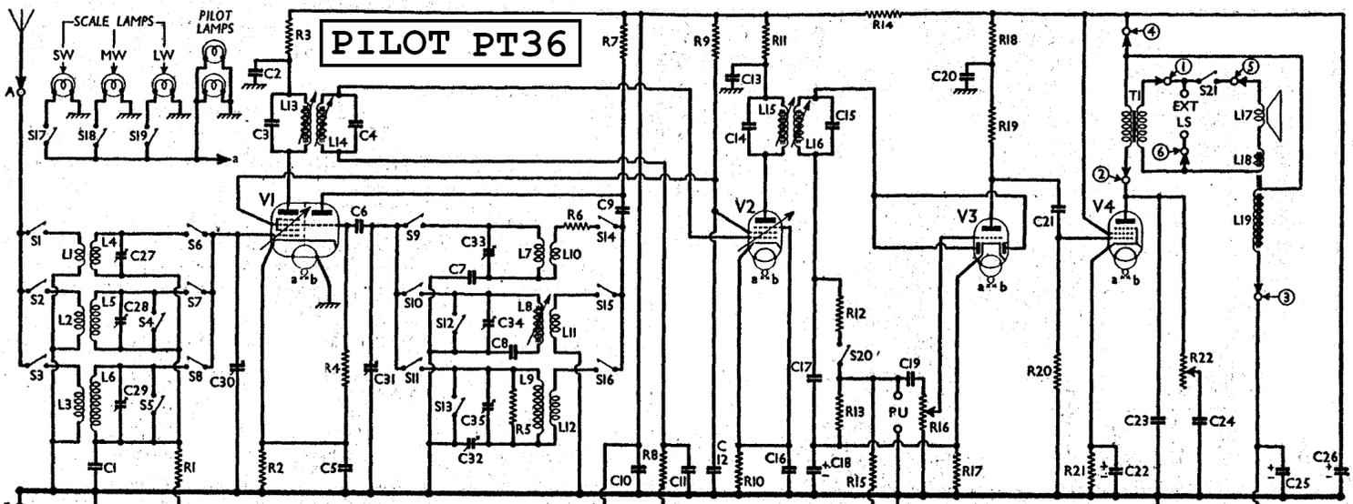
IF transformers have adjustable iron cores for tuning.
