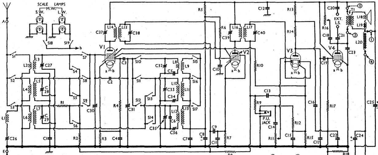
Circuit diagram of the Pilot U355 A.C. receiver. The connections of the speaker plug and socket are indicated by numbers in circles and arrows, and the socket, looking at the tag side, is inset. L1, C26, form a special filter used on L.W.
