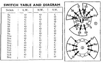
The two switch units, as seen from the front of the underside of the chassis.
