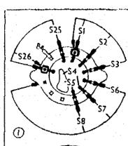
Switch unit diagrams, seen from the underside of the chassis, in the direction of the arrows in the under-chassis view. Be indicates "bearer" and Bl "blank." Note the large contact on each rotor forming extra switches.
