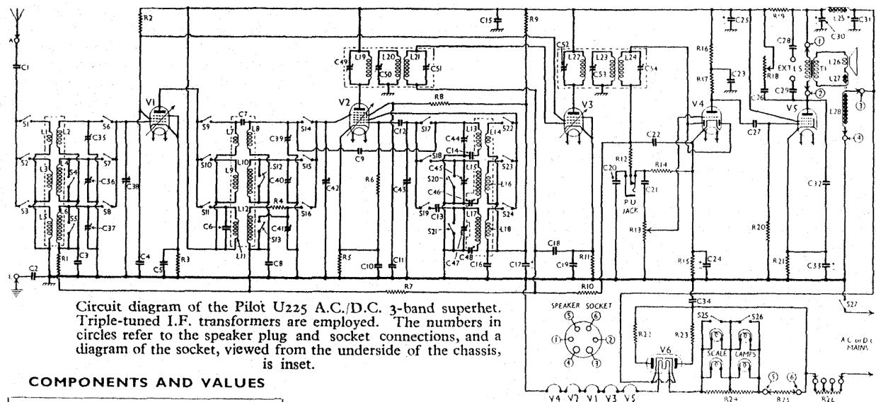
Circuit diagram of the Pilot U225 A.C./D.C. 3-band superhet. Triple-tuned I.F. transformers are employed. The numbers in circles refer to the speaker plug and socket connections, and a diagram of the socket, viewed from the underside of the chassis, is inset.
