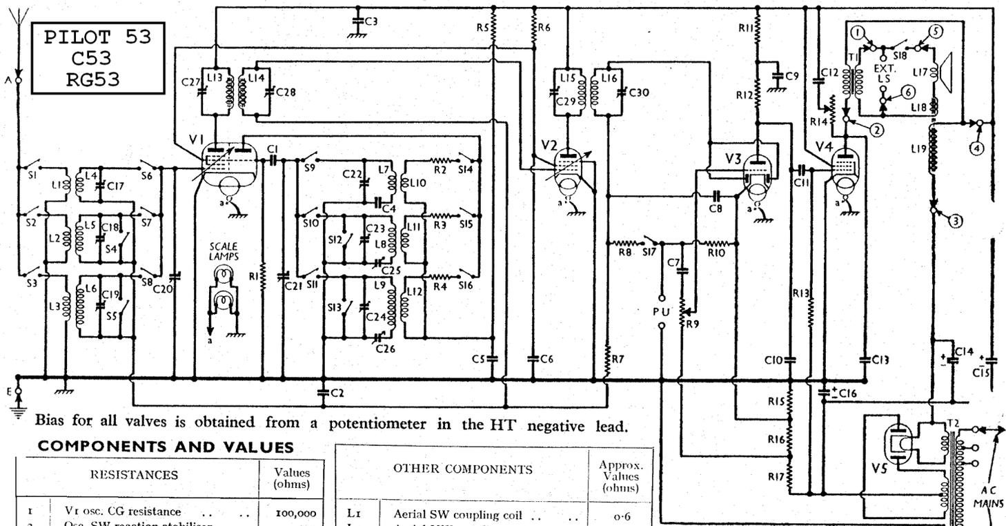
Bias for all valves is obtained from a potentiometer in the HT negative lead.
