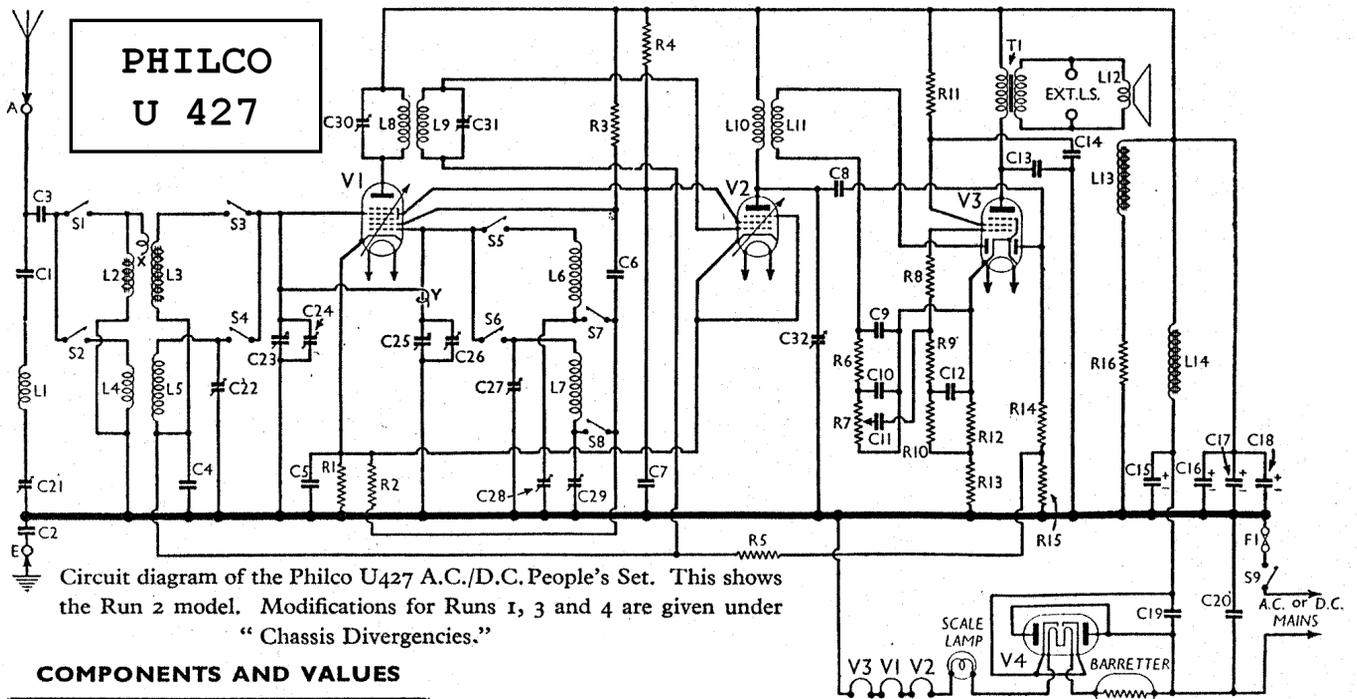
Circuit diagram of the Philco U427 A.C./D.C. People's Set. This shows the Run 2 model. Modifications for Runs 1, 3 and 4 are given under "Chassis Divergencies."
