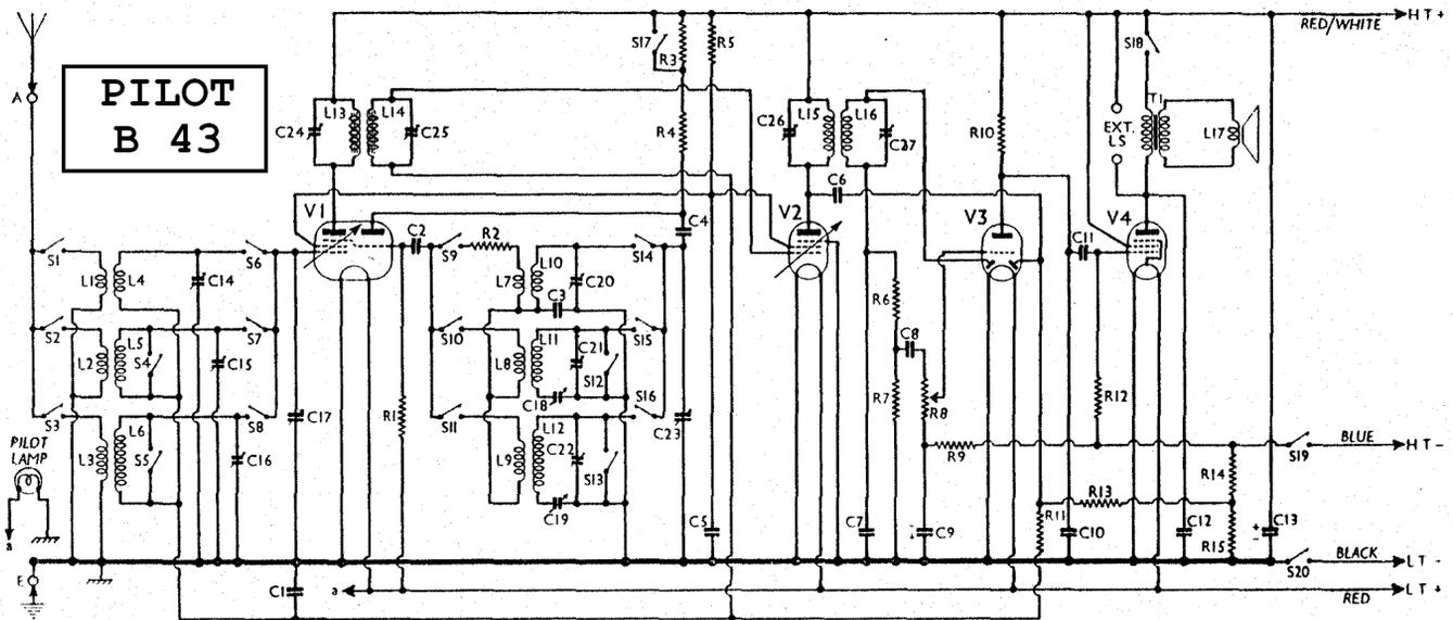
Note the automatic bias arrangements in this circuit diagram of the Pilot B43 3-band battery superhet, the potential divider **R14, R15** in the HT negative lead providing grid bias for all four valves and also delay voltage for the AVC system.
