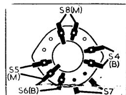
Diagram of the mains/battery change-over switch. (B) Switches close for battery operation, and (M) for mains.
