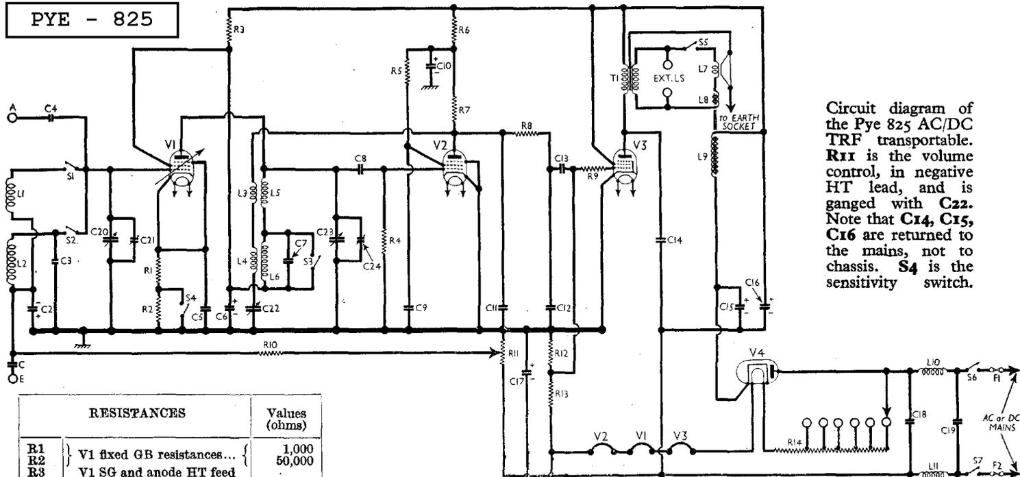
Circuit diagram of the Pye 825 AC/DC TRF portable. **R11** is the volume control, in negative HT lead, and is ganged with **C22**. Note that **C14**, **C15**, **C16** are returned to the mains, not to chassis. **S4** is the sensitivity switch.
