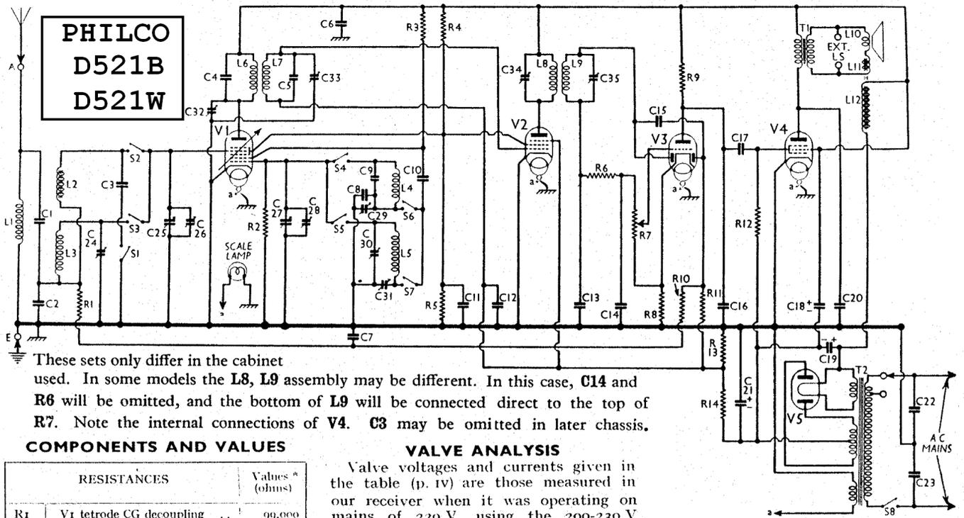
These sets only differ in the cabinet used. In some models the L8, L9 assembly may be different. In this case, C14 and R6 will be omitted, and the bottom of L9 will be connected direct to the top of R7. Note the internal connections of V4. C3 may be omitted in later chassis.
