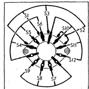
Diagram of the waveband switch unit S1-S12, drawn as seen when viewed from the rear of the inverted chassis. Below is the associated switch table.
