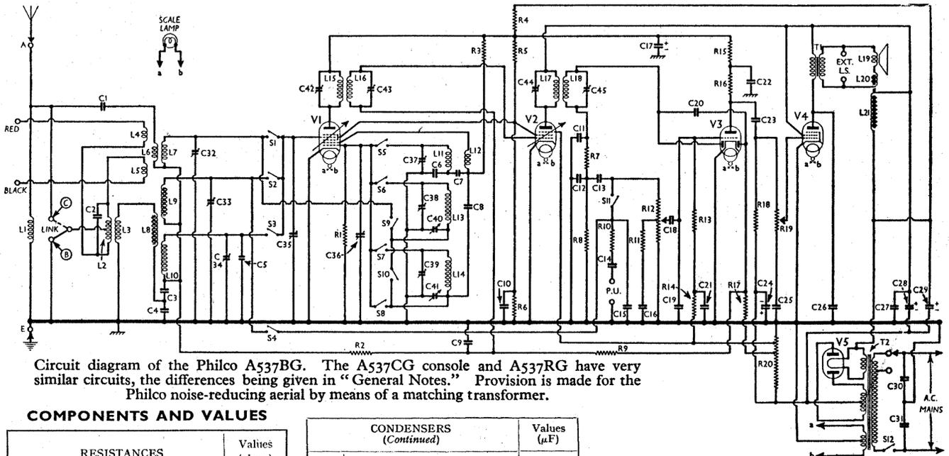
Circuit diagram of the Philco A537BG. The A537CG console and A537RG have very similar circuits, the differences being given in "General Notes." Provision is made for the Philco noise-reducing aerial by means of a matching transformer.
