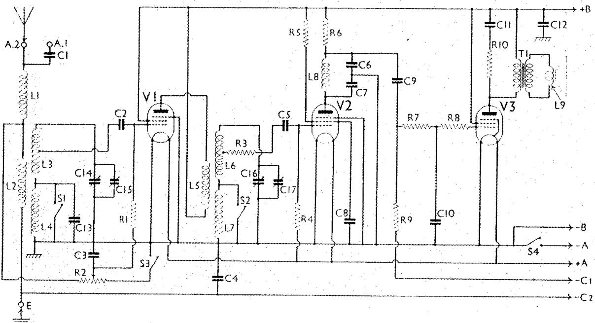
The circuit diagram of the Mullard MB3. Note that the chassis is not at earth potential. R7, R8 and C10 form a special H.F. filter. L1 is an aerial loading coil.
