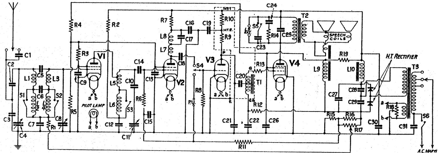
The circuit of the "Twin Supervox." The trimmers of the tuning condensers are not shown. The components in the dotted enclosure form the L.F. coupling unit, shown in Fig. 2.
