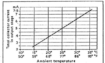
corresponding to the ambient temperature as shown on the transistor bias chart below, e.g., if the ambient temperature is 20° centigrade the corresponding current reading for correct quiescent bias is 3.75mA.
