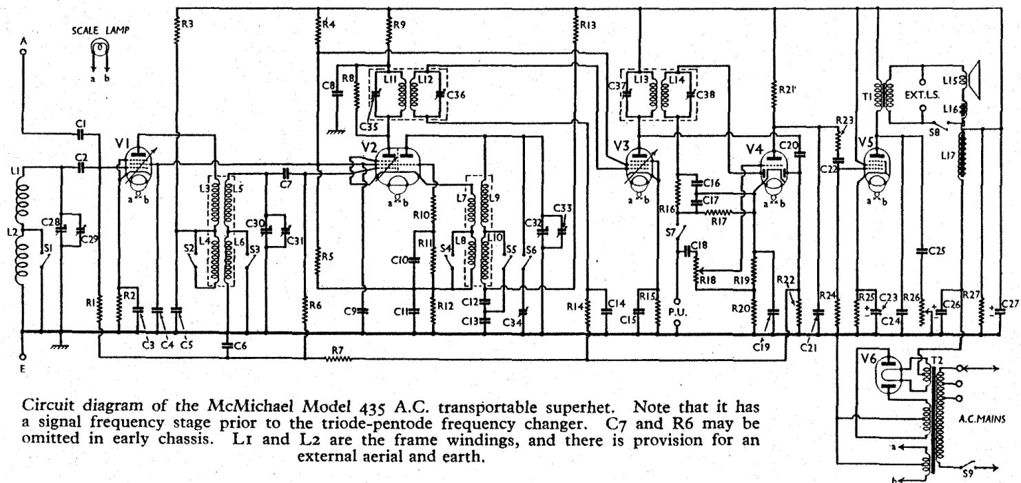
Circuit diagram of the McMichael Model 435 A.C. transportable superhet. Note that it has a signal frequency stage prior to the triode-pentode frequency changer. C<sub>7</sub> and R<sub>6</sub> may be omitted in early chassis. L<sub>1</sub> and L<sub>2</sub> are the frame windings, and there is provision for an external aerial and earth.
