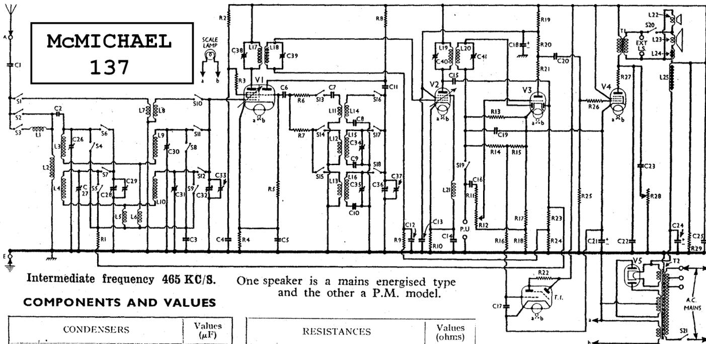
Intermediate frequency 465 KC/S. One speaker is a mains energised type and the other a P.M. model.
