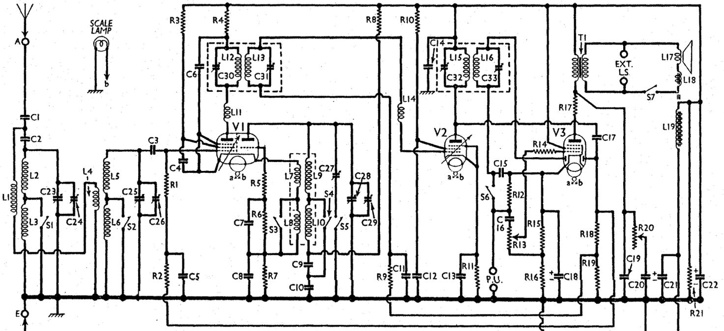
Circuit diagram of the McMichael 235 A.C. superhet. A conventional circuit is used, with a triode-pentode frequency changer and a double diode output pentode valve. Pick-up and external speaker connections are made via the usual McMichael jack sockets, shown on the diagram as switches S6 and S7.
