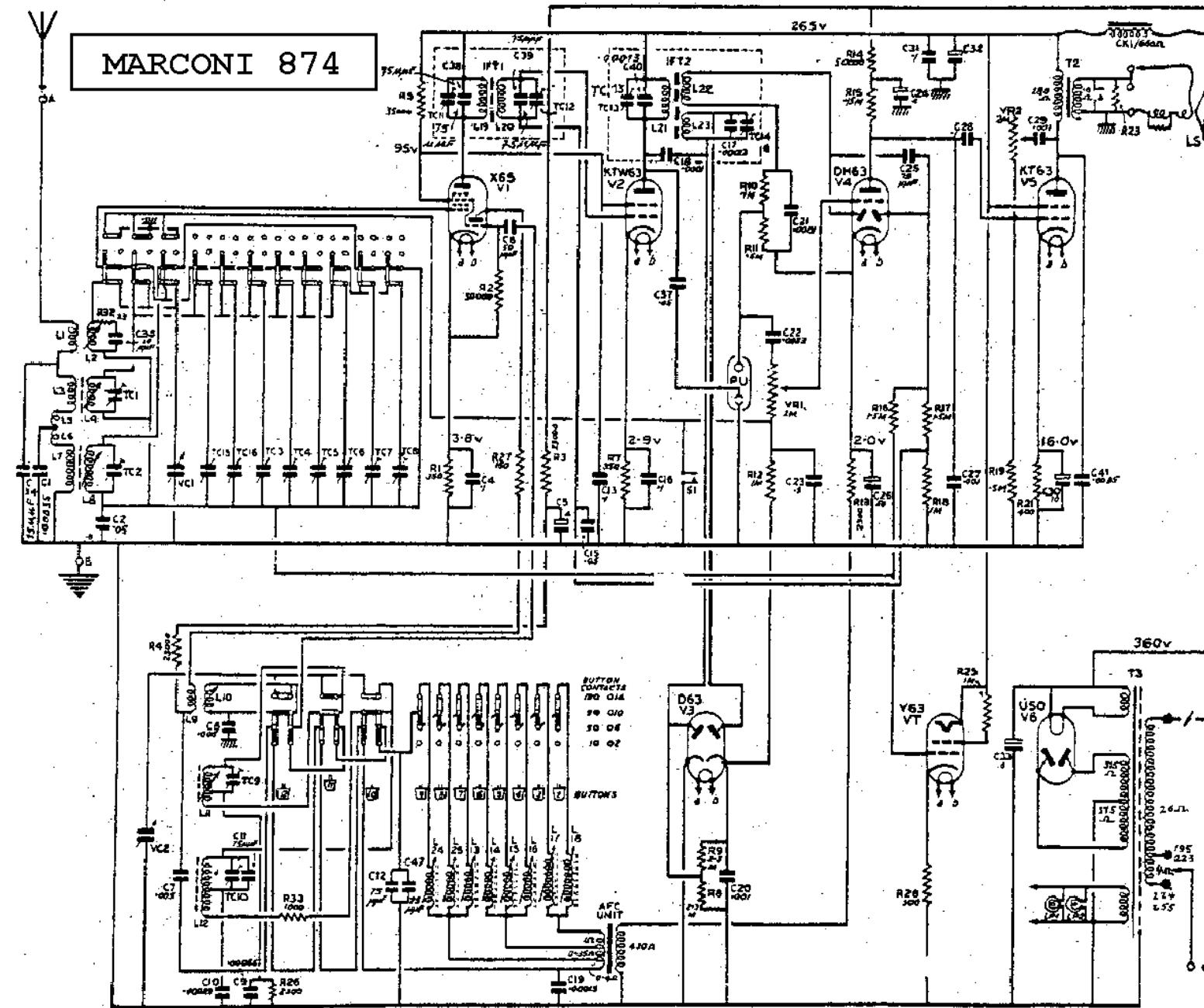
The push button switch is shown with MW button pressed.
