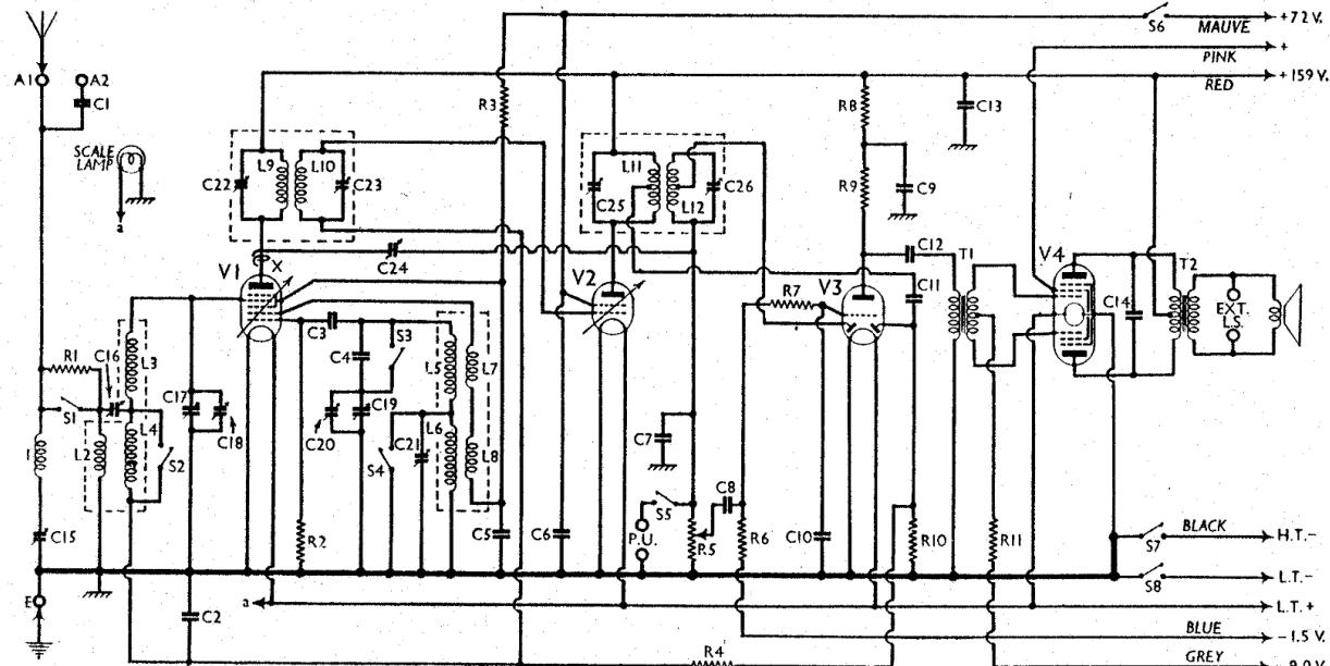
Circuit diagram of the Marconi-phone 234 battery superhet. The earlier Model 257 has a similar circuit. X is a small coupling, providing I.F. reaction, controlled by C24. The H.T. voltage of the pink lead depends on the letter marked on the bulb of V4. (See General Notes.)
