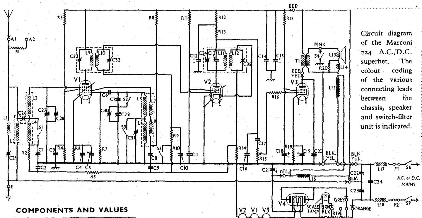
Circuit diagram of the Marconi 224 A.C./D.C. superhet. The colour coding of the various connecting leads between the chassis, speaker and switch-filter unit is indicated.
