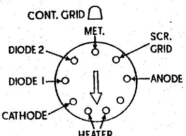
Connections of V<sub>2</sub>, a double diode H.F. pentode, looking at the underside of the base.
