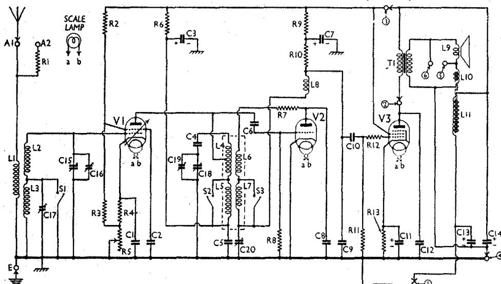
The circuit diagram of the Marconiphone Model 235 A.C. receiver. Note the aerial series resistance in place of the more usual condenser. The small figures in circles denote the connections between the speaker chassis and the main chassis. Between tags 4 and 5, that is, in parallel with the hum neutralising coils L<sub>10</sub>, is connected a small length of resistance wire, not shown in the circuit diagram.
