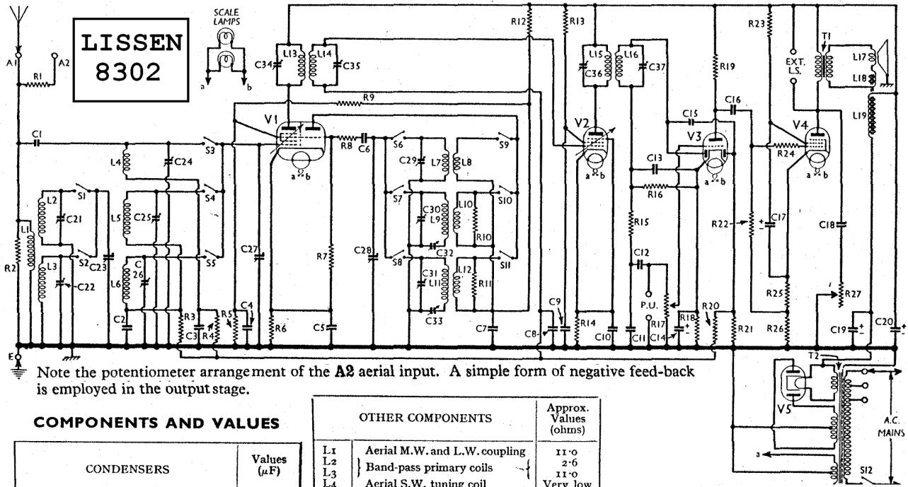
Note the potentiometer arrangement of the A2 aerial input. A simple form of negative feed-back is employed in the output stage.
