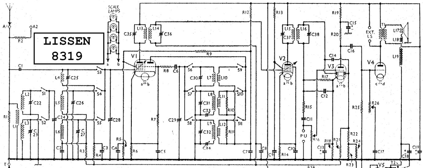
Note that a triode output valve is used, its filament being run from a separate secondary winding on T2.
