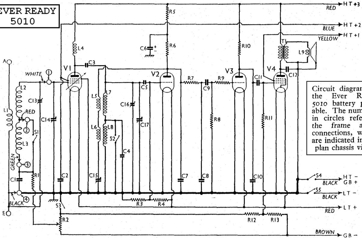
Circuit diagram of the Ever Ready 5010 battery portable. The numbers in circles refer to the frame aerial connections, which are indicated in the plan chassis view.
