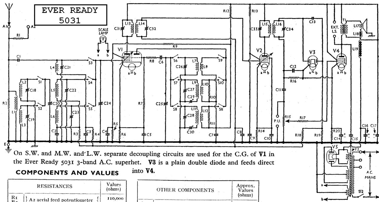
On S.W. and M.W. and L.W. separate decoupling circuits are used for the C.G. of **V1** in the Ever Ready 5031 3-band A.C. superhet. **V3** is a plain double diode and feeds direct
