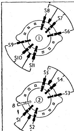
Diagrams of the switch units, as seen looking in the direction of the arrows in the under-chassis view on page III.
