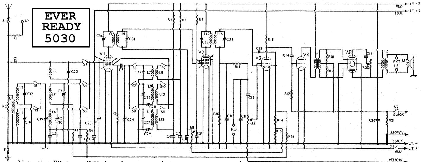
Note that **V2** is an R.F. hexode, connected to operate as a pentode.
