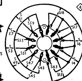
Circuit diagram of the Ekco A52. The connections which need to be unsoldered to remove the group of R.F. and oscillator components as described under "Dismantling the Set" are indicated by arrows and solid circles and numbered 1-22. The waveband indicator lamp is connected to the heater circuit via the contact plate.
