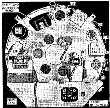
Rear view of the chassis, showing all the valve positions, **V4** being on the horizontal deck. The cover has been removed from the scale lamp inspection hatch, and the lamp and cursor are seen through the aperture.
