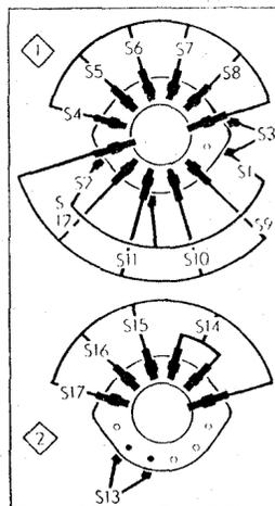
Diagrams of the waveband switch units, as seen when viewed in the direction of the arrows in our plan view above.
