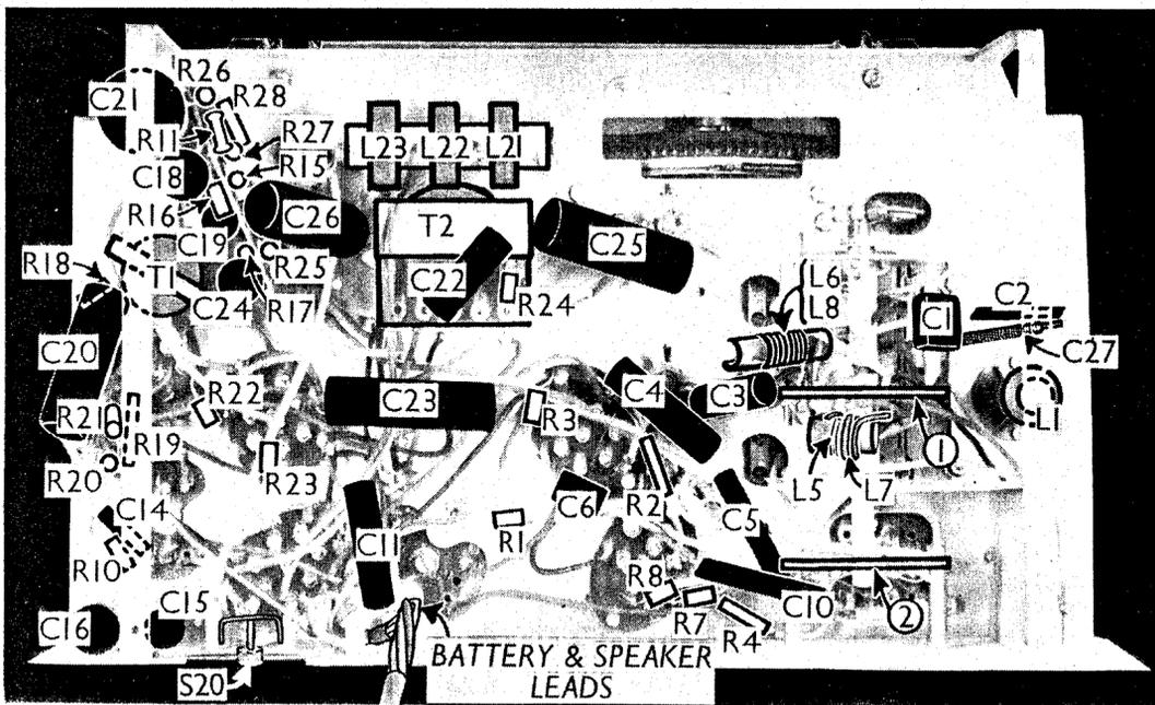
Under-chassis view. C27 is a small semi-variable condenser. The core of L1 is adjustable through a hole in the chassis deck. Diagrams of the switch units are on the back of this sheet. L5 and L7 are the aerial coils for the television sound band.
