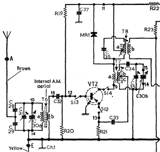
Diagram of the switch unit. Transistors are connected to the moving contacts as shown.
