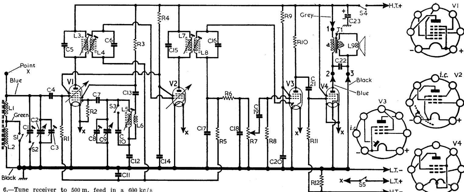
6.—Tune receiver to 500 m, feed in a 600 kc/s signal and adjust the core of L5 (A2) for maximum output while rocking gang for optimum results.
