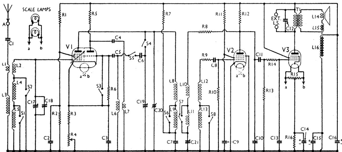
Circuit diagram of the Cossor 3783 3-band A.C. receiver. It operates as a simple superhet on the S.W. band only, the circuit on M.W. and L.W. being that of a 3-stage T.R.F. model.
