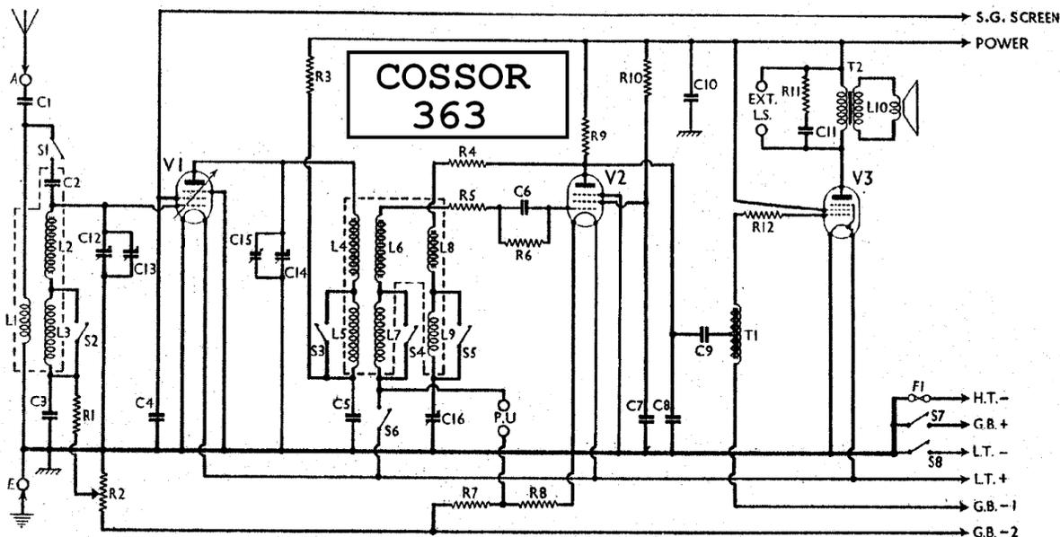
Circuit diagram of the Cossor Model 363 battery receiver. The M.W. coils are iron-cored. The circuit is quite straightforward, volume being controlled by varying the bias of V1.
