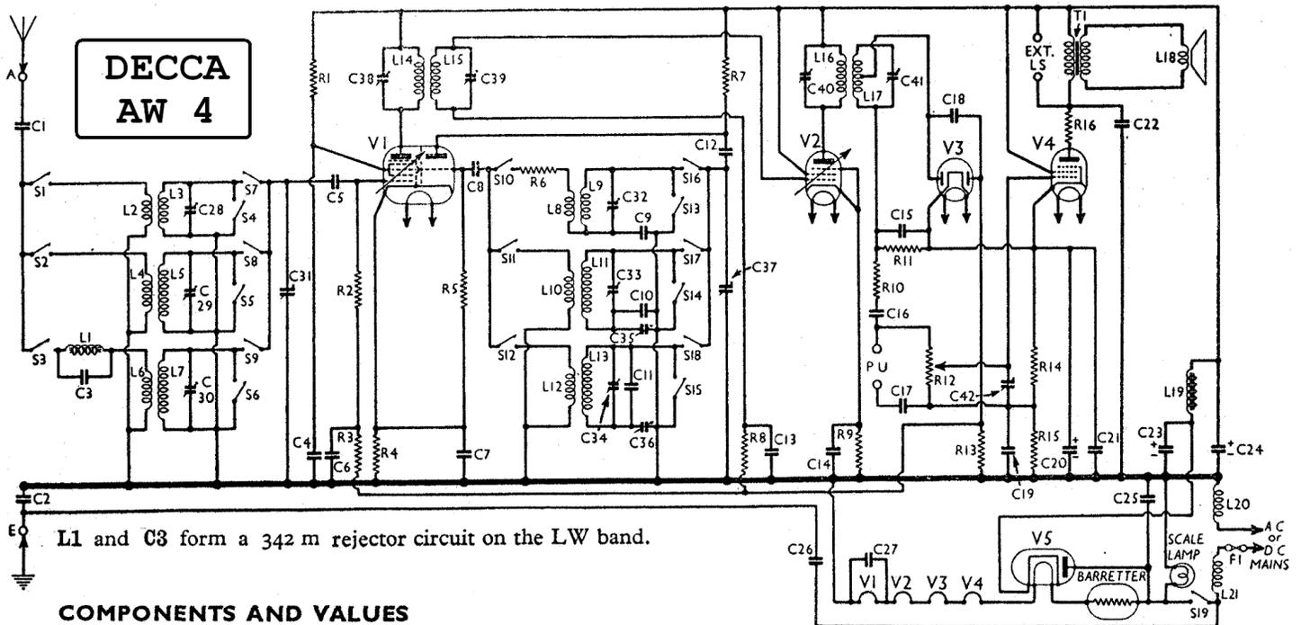
L1 and C3 form a 342 m rejector circuit on the LW band.
