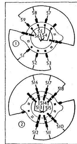
Switch diagrams, looking in the directions of the arrows in the under-chassis view.
